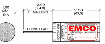
Dimensions are in Inches Dimensional Tolerances: ± .03 (.76mm) (Metric equivalents in parenthesis)
