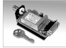
This Chassis Mount Kit provides a convenient package to use any CA Series precision high voltage power supply without having to fit it onto a PC board. The Kit also provides for easy prototyping and evaluation. Extra filtering on the input and output improves performance. A schottky diode on the input provides reverse polarity protection. Input connector is via a 15P SUB MIN-D plug (mate supplied) and output is via an MHV style coaxial connector (mate supplied).
